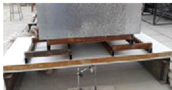
**B:** a device model of quadruple concentrated loading samples
