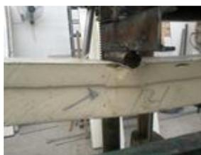
**d:** - a sample figure shows the local distortion happened when the collapse takes place with separation of the core's material.
