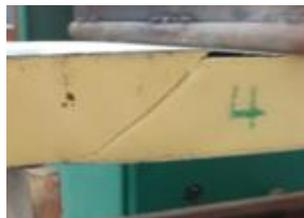
**c:** shearing collapse of the core in a 45degree angle.
