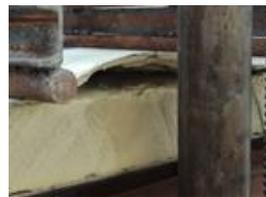
**b:** a sample figure explains rupture of the core and separation of the layer between the two points of applying load.
